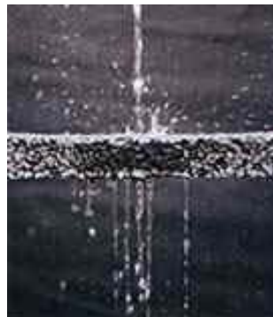
Figure 4.3 Cross-Section of Pervious Concrete
